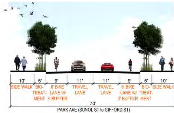
Figure 5.1.4: On-Street Primary Bicycle Facility
