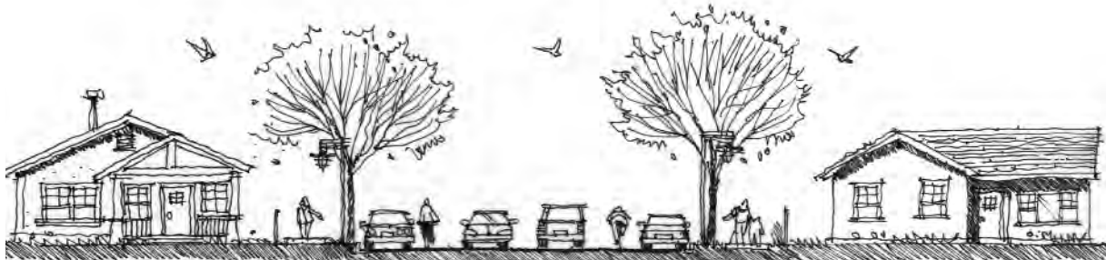
Conceptual section of potential Scott Street improvements with sidewalks, bike lanes, lighting, landscaping and route signage.
